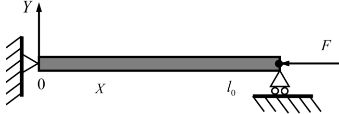
Figure 4.1 Model of a simply-supported inflatable beam subjected to axial compression load.
