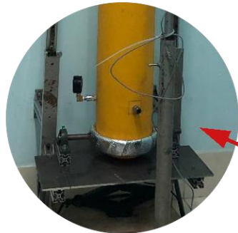
Figure 5.24 The fixed-end and pin-end support
