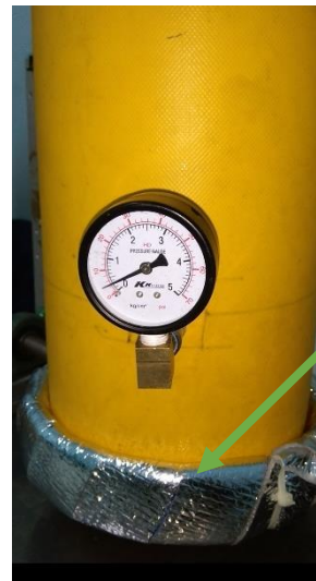
Figure 5.27 The locator ring can be adjusted in diameter
