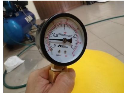
Figure 5.21 Inflatable beam's manometer
