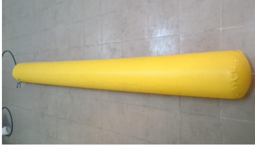
Figure 5.20 Inflatable beam after pumping
