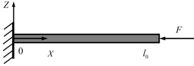
Figure 4.3 Model of a cantilever inflatable beam under axial compression load.
